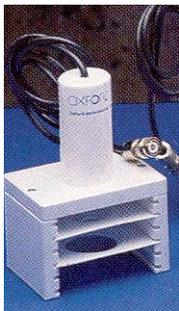
This is the Geiger-Mueller tube (Cylindrical Object at the top) and the stage. The stage holds the sample carrier and radioactive source.
