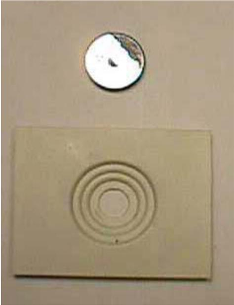
This is the sample carrier and a Radioactive source.
