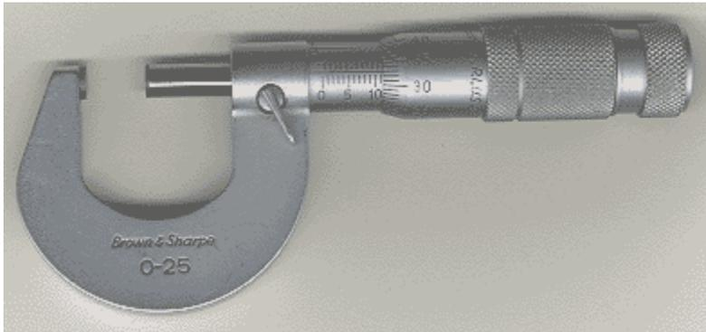
Figure 1 0-25 millimeter micrometer
