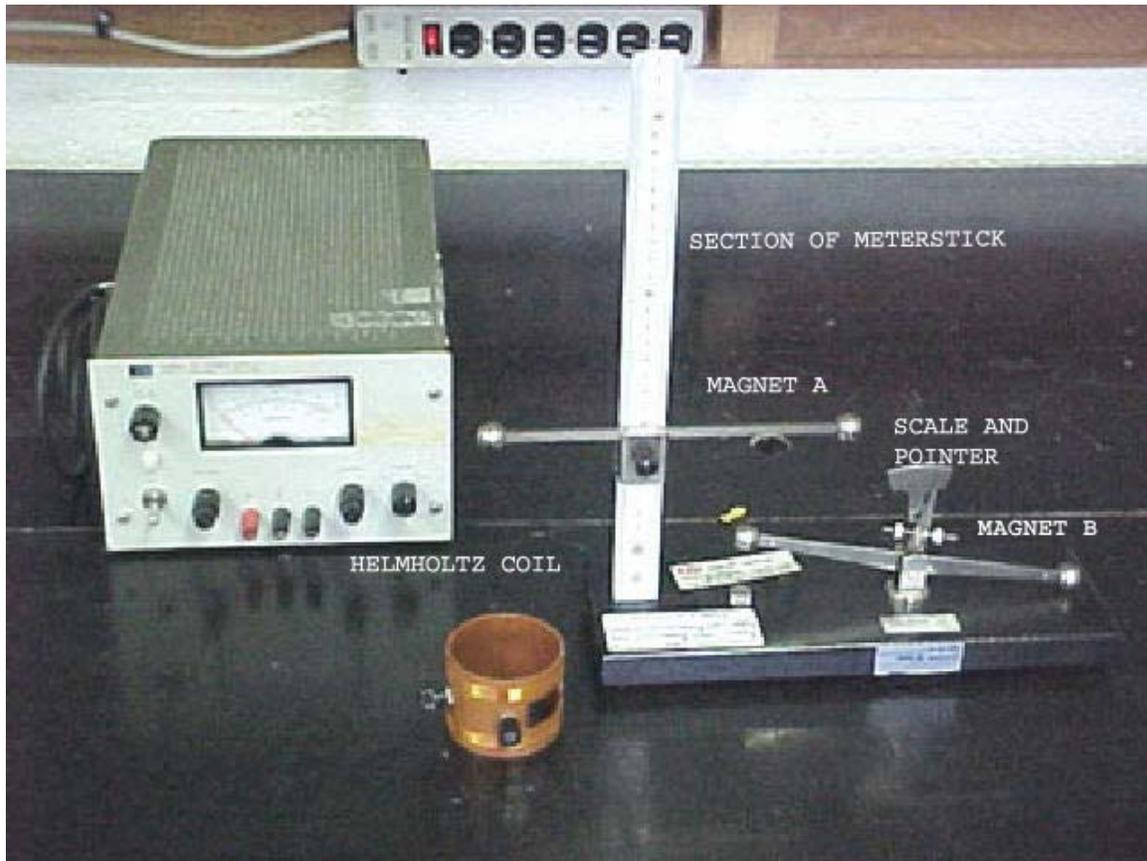
Our setup will look almost the same as this one. We will use the DC wall outlets to put a current through the Helmholtz coil instead of a separate stand alone power supply.
