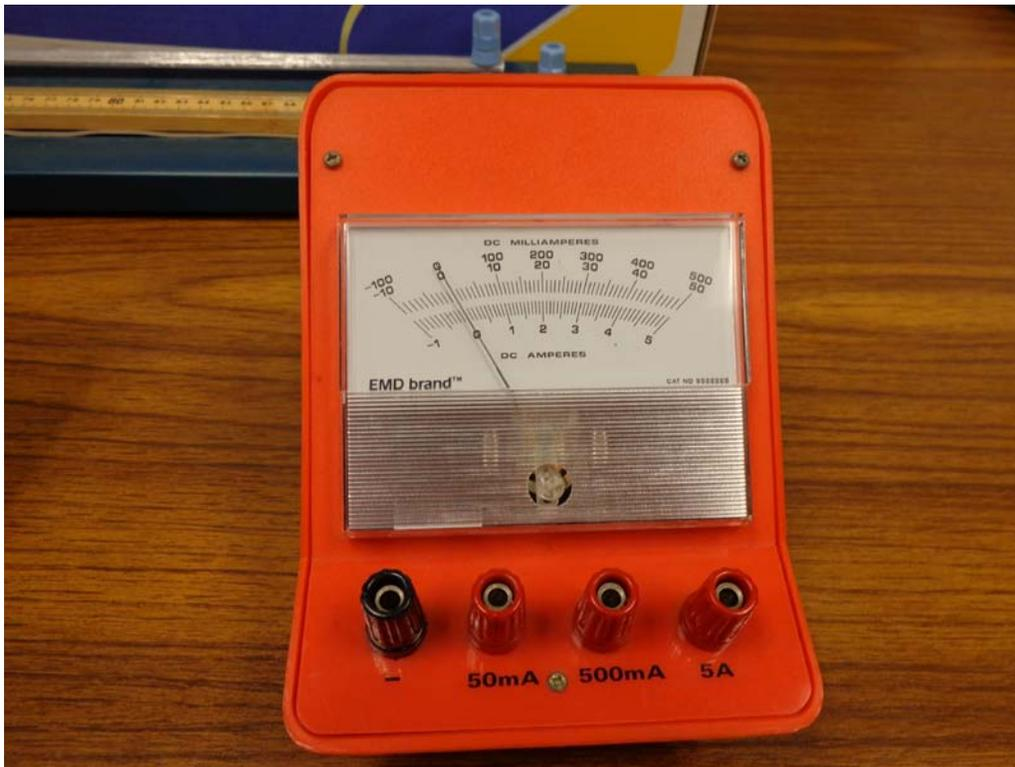
Figure 4: Three Range Ammeter. Note the three different Red (+) connectors and the Black (-) output. Also note the three different scales that match the three Red connectors.
