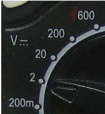
**2. Manual experiment: Record the value of the resistor in the data table. Measure the current for 12 different voltages, with the increment of 1V (See Fig. 8). Record the current and voltage in your data table. Record the instrumental error in your measurements. The instrumental error is taken as  $\pm 1/2$  of the smallest division on the scale of the analog device, and  $\pm 1$  in the lowest digit for the digital device.**
