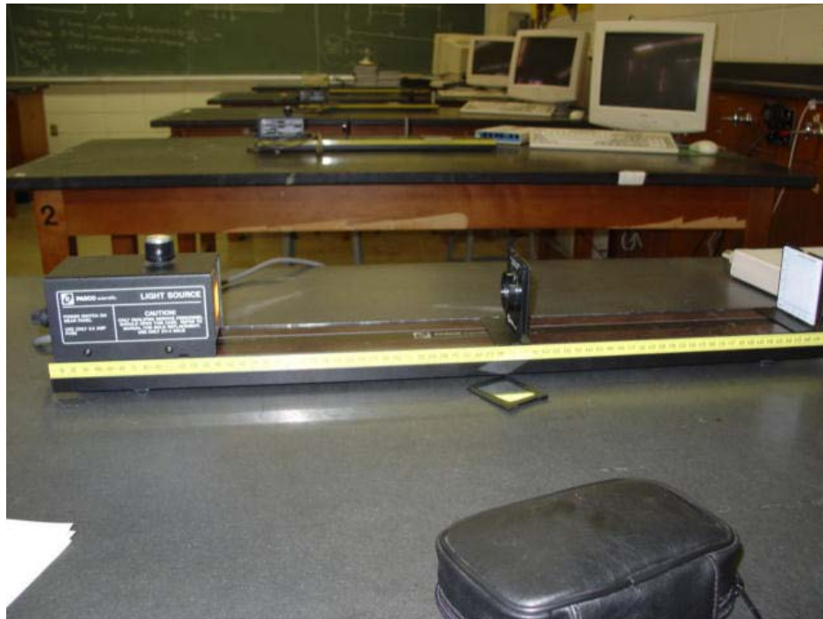
Figure3. Optical Bench with Light Box, Lens, Screen.
