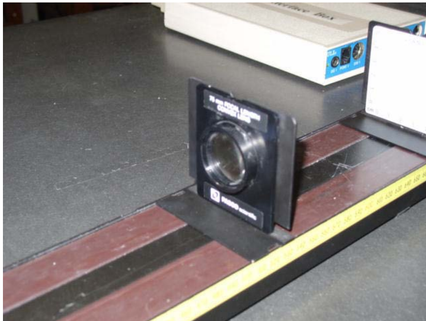
Figure 6: Lens attached to Lens mount. Note: the lens must be mounted on the lens mount on the side of the mount where the metal foot has been cut. See figure 7.
