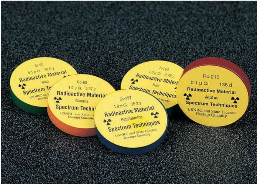
**Figure 4: Different Radioactive sources. Note the Activity, Half Life of each and the radioactive particles emitted.**
