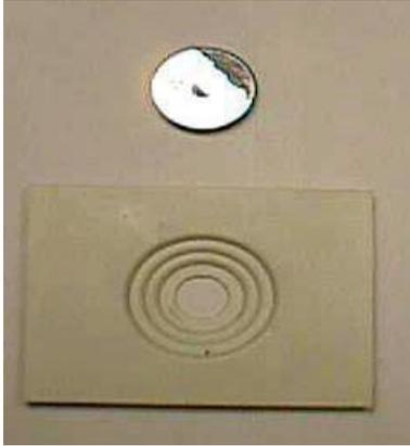
**Figure 3: Radioactive source and sample carrier.**
