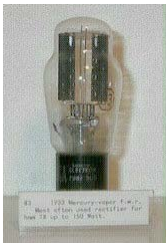
1933 RCA 83 Full Wave Rectifier with mercury vapor. This tube is equivalent to our circuit,
