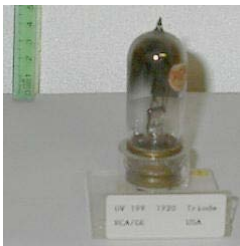
1920 RCA UV199 Triode The first from RCA to be machine manufactured.
