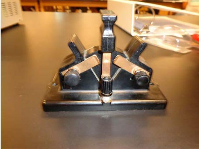
Figure 7: Double Pole Double Throw Switch
