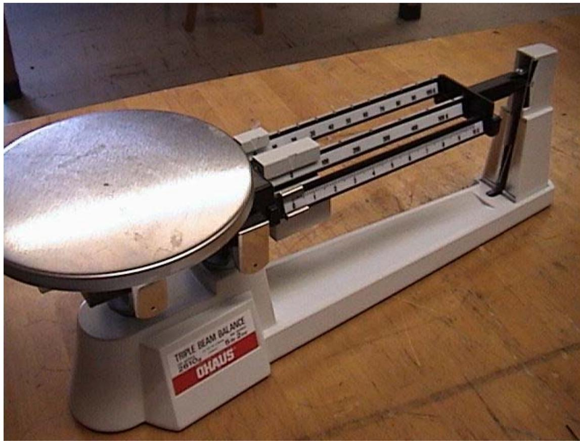
Figure 2 Triple Beam Balance
