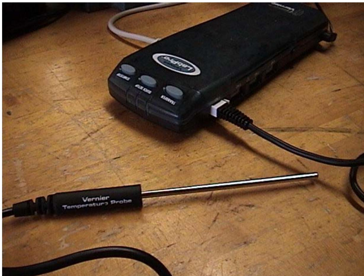
Figure 1 Vernier LabPro Interface and Stainless Steel Temperature Probe
