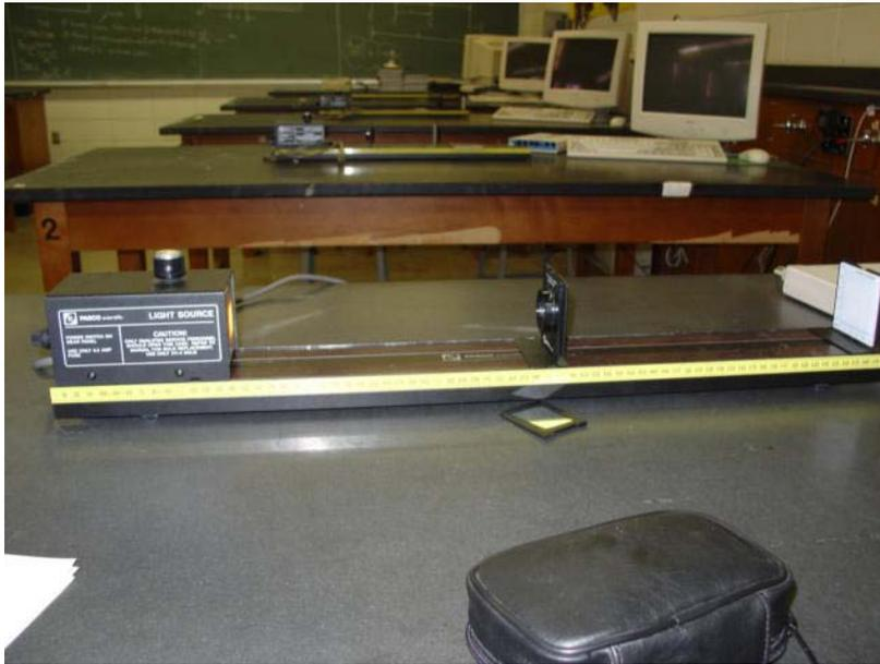
**Figure 2. Optical Bench with Light Box, Lens, Screen.**
