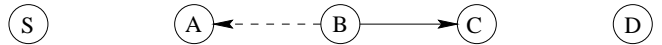
Figure 2: When B forwards a packet from S toward D through C, A can overhear B's transmission and can verify that B has attempted to pass the packet to C. The solid line represents the intended direction of the packet sent by B to C, while the dashed line indicates that A is within transmission range of B and can overhear the packet transfer.
